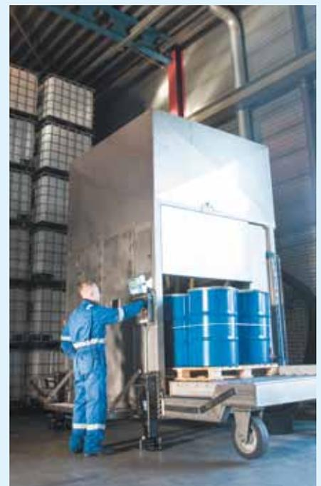
enables filling to take place in a fully protected area, which improves safety. By means of a powered roller conveyor, the pallets (carrying jerry cans or drums) or IBCs are automatically moved to or from the filling line. Filling does not start until all holes have been detected and all doors are closed.
